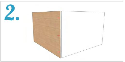
Line up spine and side panels with holes to create 90 degree corner, and start all 3 bolts by hand until threads are engaged. Once engaged, tighten with cordless. Once complete, fasten the bolts tight and ensure both panels are level. Use levelers to adjust.
