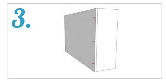
Line up 24" return panel with holes at end of side panel and start all 3 bolts by hand until threads are engaged. Once engaged, tighten with cordless. Once complete, fasten the bolts tight and ensure both panels are level. Use levelers to adjust.
