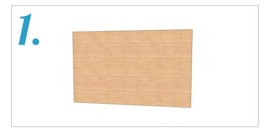
Place first spine panel, and ensure it is level. Use levelers to adjust if needed.
